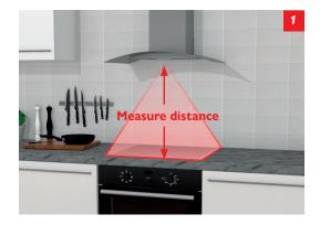
Measure the installation height. The Heat Sensor should be centred above the cooker, preferably within Zone 1 (see diagram at bottom of the page). It can be attached to the grease filter. It is also important to ensure the minimum distance from any lights underneath the hood is 10 cm (5 cm is enough for LED lamp).
